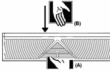
2.) Support diffuser by its top as shown with one hand (A) entering the bottom with the other hand (B)
