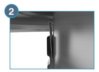
2. Press firmly until the locking tabs snap into place below the curled inner edge of pipe
