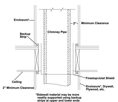
Figure 7 Firestop/Joist Shield with Full Enclosure
