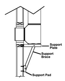
Figure 2 Wall Support for 10" and 14" Chimneys
