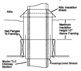
Figure 6 Firestop/Joist Shield used with Attic Insulation Shield
