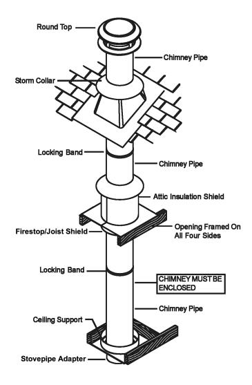
Figure 1 Vertical Chimney through One-Story and Attic
