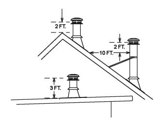
Figure 4 Rules for Chimney Height above the Roof
