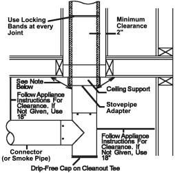
NOTE: The purpose of the diagonal arrows is to show that the 18-inch clearance DOES NOT APPLY to the vertical connector entering a support. This support is actually tested with a bare vertical connector and must pass the UL tests with very hot gases entering the bare single-wall pipe.
