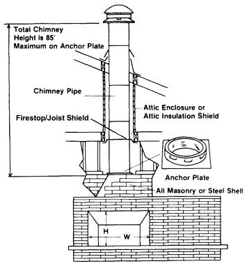
Figure 5 Anchor Plate Support for Mason Fireplace
