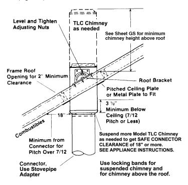
Figure 3 Required Clearances for Roof Support
