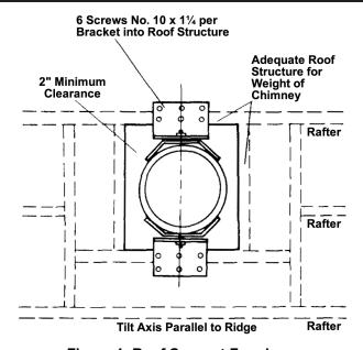
Figure 1 Roof Support Framing
