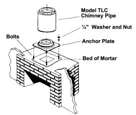
Figure 4 Anchor Plate Installation in Masonry Fireplace
