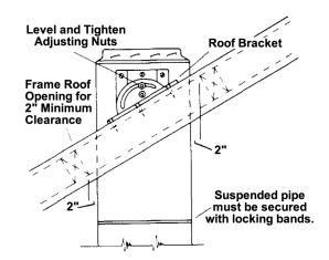
Figure 2 Roof Support Position on Sloped Roof
